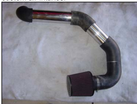
Custom ductwork and air filter ready to be installed in a vehicle.
