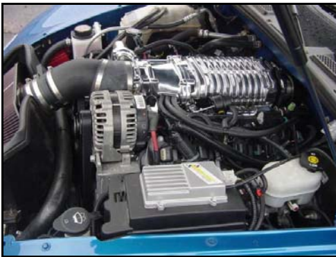
SSR with a new Supercharger
