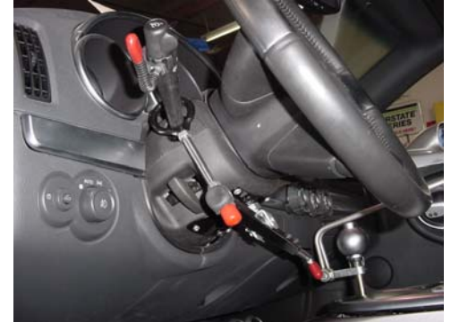
"Knee" Controls to operate turn signals
